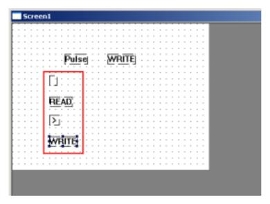
11、Modify "READ" unit's property, its object is PSW300, modify "Write" unit's property, its object is PSW300, Set data as 0. Modify compare unit's right operand as 59. Choose the four units, open its advanced property.
