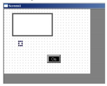
8、Add a write unit, modify its type as register, the object as PSW300、Set data as 1. Copy one, set its data as 0
