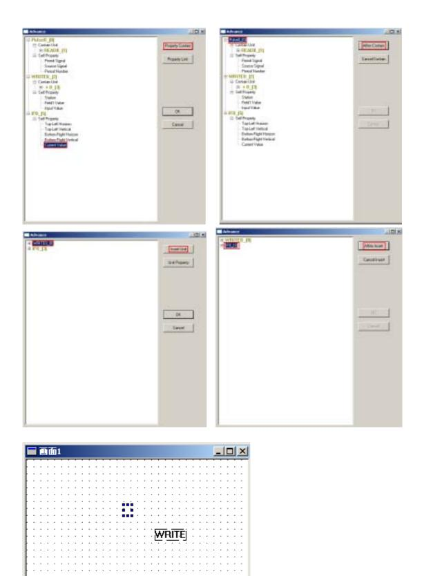
15、Finish the interior operation, let's make the alternate interface. Add a "Text" and a "Digital display" unit in the screen, modify the display unit's content as "Second", digital display's object
