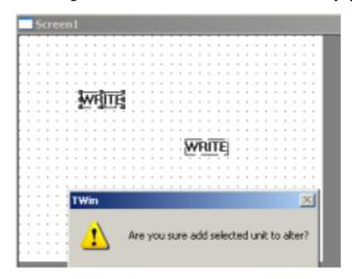
17、Now we finish the interior process of compare operation. Now let's make the alternate interface. Add a "Text" unit in the screen, two "Digital Input" units, one "Digital Display" unit. Modify the text display content as "Please enter two values: (The larger is been put out), modify two "Digital Display" units, make their object separately point to PSW300 and PSW301, modify "Digital Display" unit's object to point PSW302. See the following chart:
