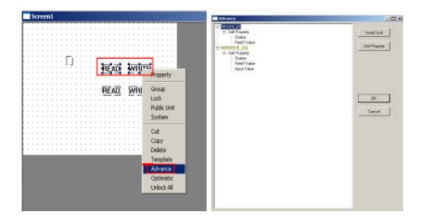
15、Choose "Write" unit WRITEO\_(0): "Input Value"→click "Property Contain"→choose READO\_0→ click "Affirm Contain"—OK. The action is to write value in PSW300 to PSW302 Do the same operation with the left READ unit and Write unit, the action is write the value in PSW301 to PSW302
