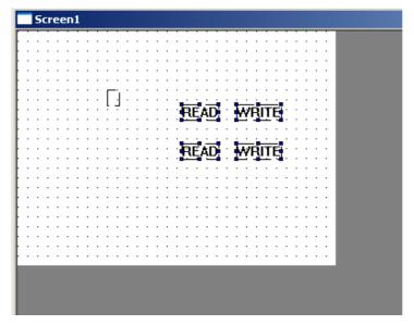
12、 Modify two "Write" units' property, the type is register, object is PSW302, see the following chart.
