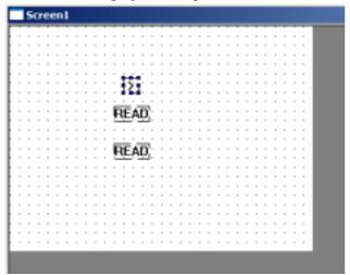
2. Modify the property of first "Read", see the following chart. Here the modify type is register, object is PSW200. Modify the second "Read", make it point PSW301.
