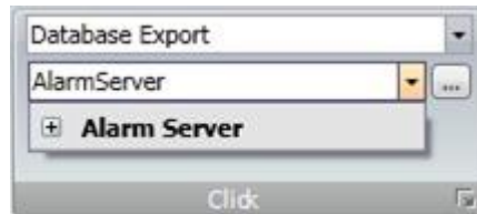
Figure 20-1. Individual Database Tables May be Selected for Export By Clicking the + Sign
