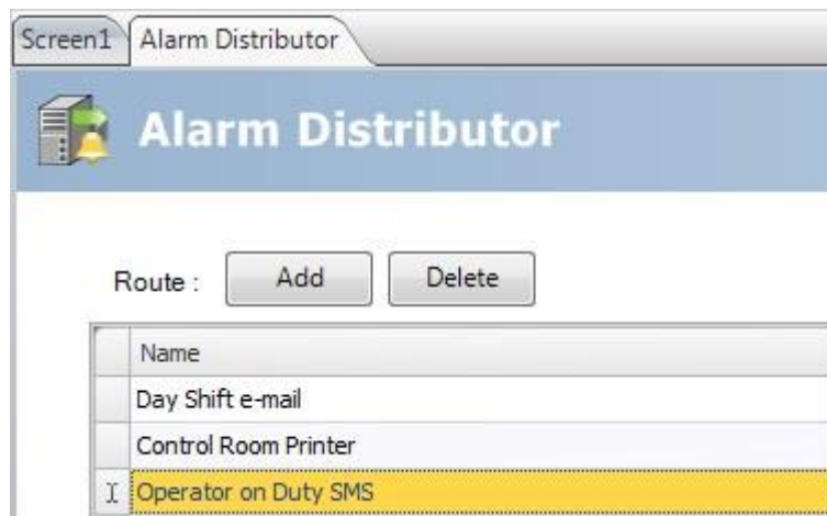
Figure 15-11. Alarm Distributor Tab
